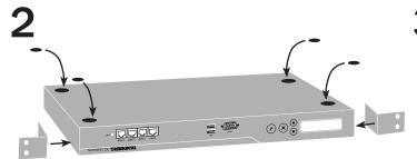
Mount the rack ears and/or rubber feet, if applicable, and turn the unit back on its feet or mount it in the rack.
